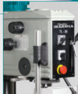
Controls mounted on the front of the headstock for operator convenience for fast and easy speed selection
